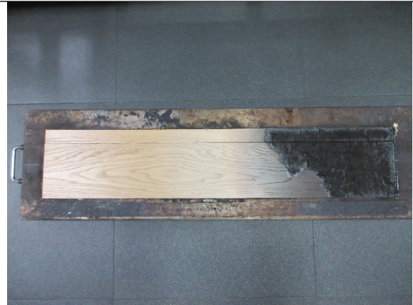
After test- Radiant heat source
